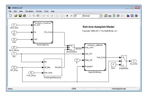
This model represents a basic roll axis autopilot with two operating modes: roll attitude hold and heading hold. The mode logic for these modes is external to this model. The model architecture represents the heading hold mode and basic roll attitude function as referenced models. The model includes:
