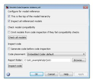
**c** Run the model compatibility checks by clicking **Check all models**. The compatibility checker displays a progress bar.
