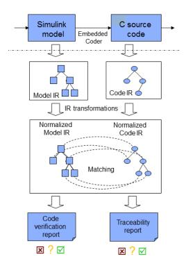
Use of normalization techniques allows the Code Inspector to inspect code generated by an highly-optimizing code generator. The results of this matching process are reported to the user by means of a code verification report and a traceability report. When code inspection completes, the code verification report documents the translation validation process, and the traceability report provides a bidirectional mapping between model elements and their counterparts in the generated code.
